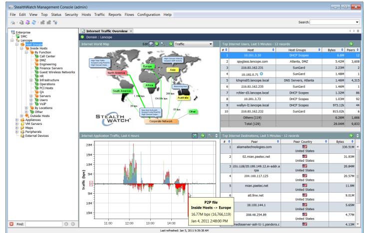
With customizable views and powerful drill-down capability, the SMC is the control center for network and security operations, performance management, traffic accounting, interface usage and user identity tracking.
